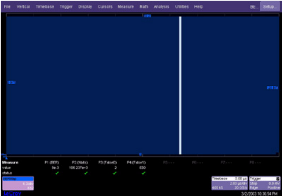
Figure 17. Bit Error Map for 127-Bit Pattern Containing Pattern Dependent Errors
