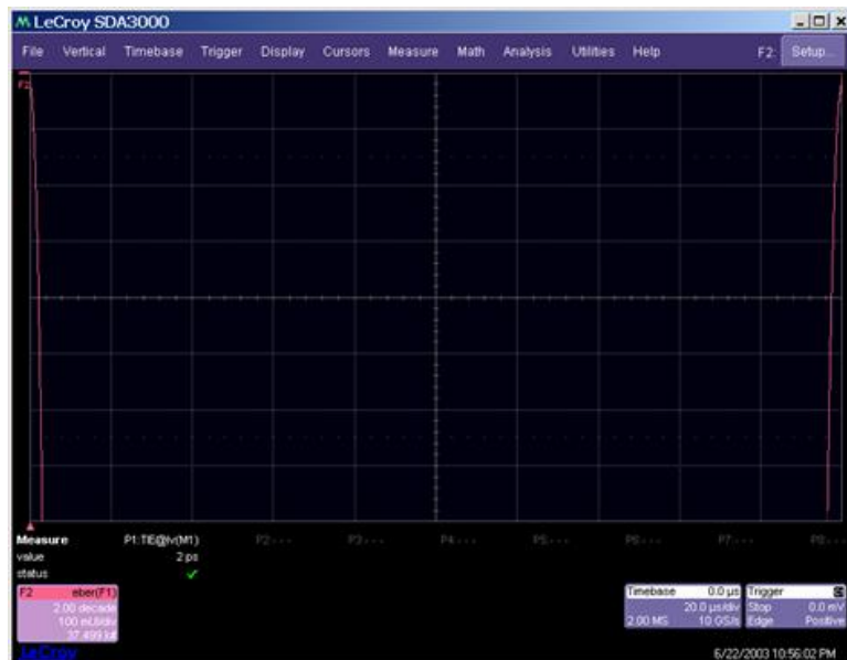
Figure 10. The bathtub curve is constructed by rescaling the total jitter curve in Figure 9 to one unit interval, and centering the right side of the total jitter curve at 0 UI and the left side at 1 UI (the left and right sides of the bathtub curve).
